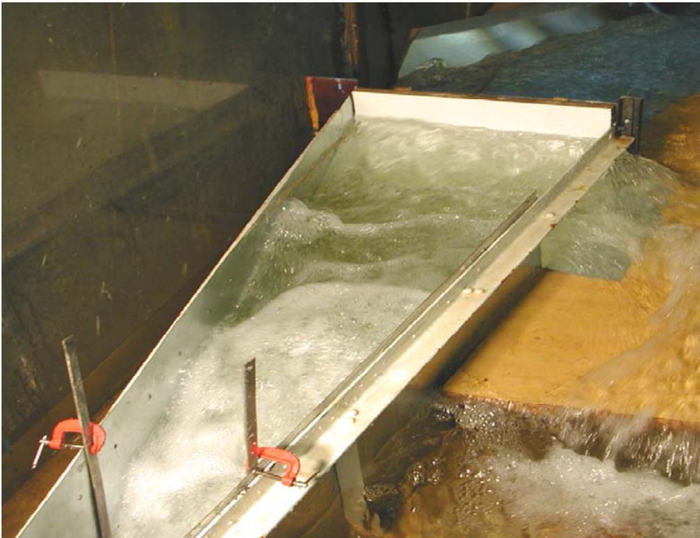
**Fig.9.** Stilling pool with the side notch operation in the case of spatial conjunction of races at  $Q=25,10 \text{ l/s}$  (design discharge).
